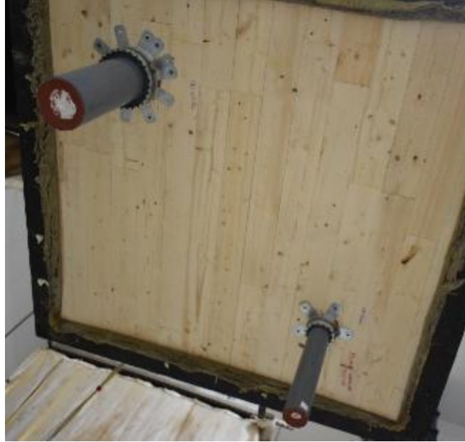
Exposed Side Before Fire Endurance
