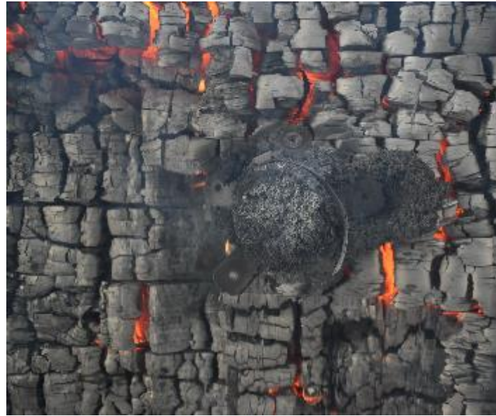
Exposed Side Post Fire Endurance, 50mm Pipe
