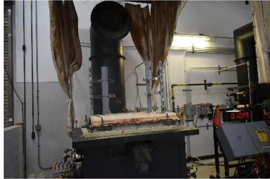
Nonexposed Side During Fire Endurance
