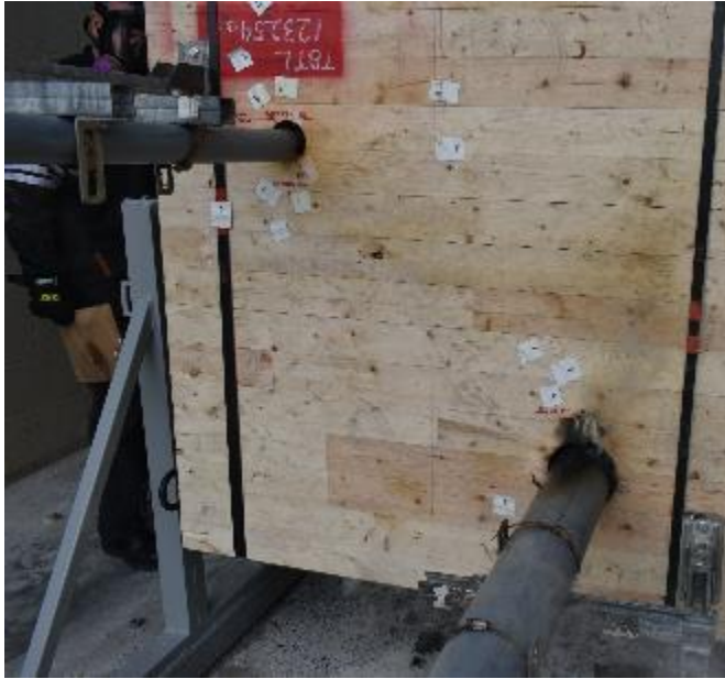
Nonexposed Side Post Fire Endurance
