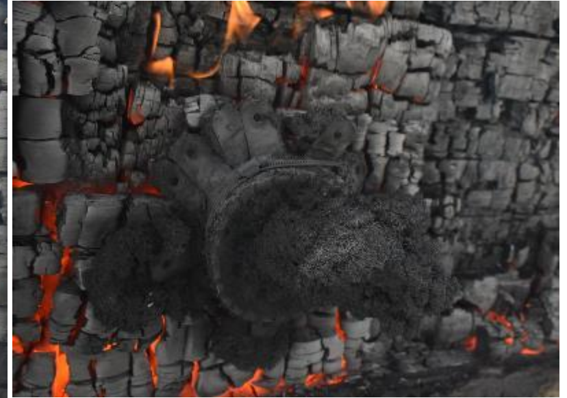
Exposed Side Post Fire Endurance, 102mm Pipe
