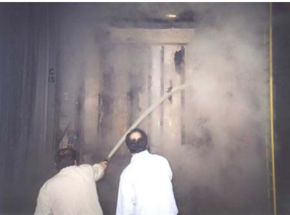
A vertical specimen is subjected to a hose stream test.
