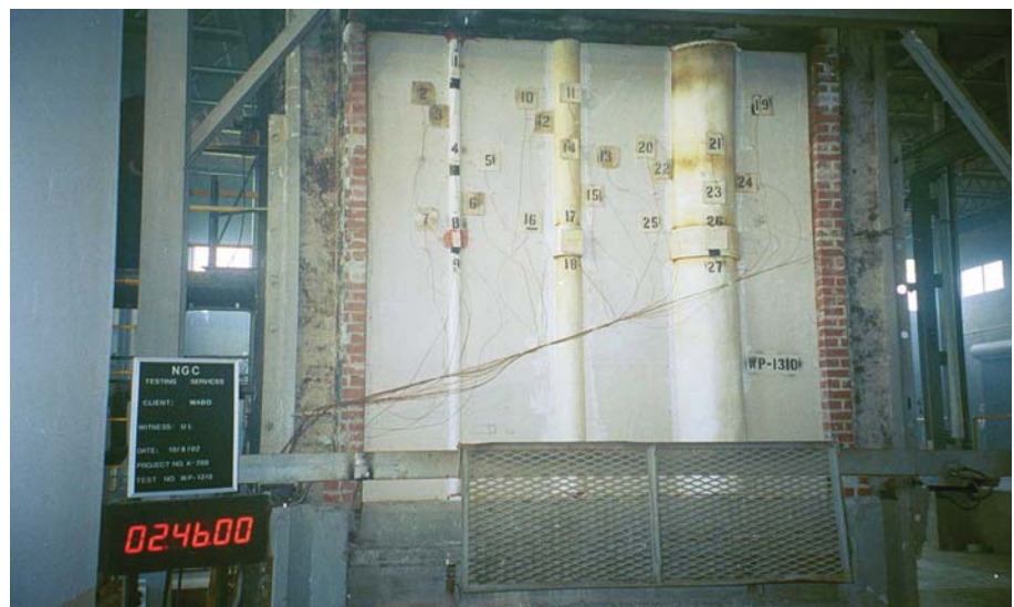
Test specimens have a minimum exposure to fire of generally 12 ft. for horizontals (top) and 9 ft. for verticals.
