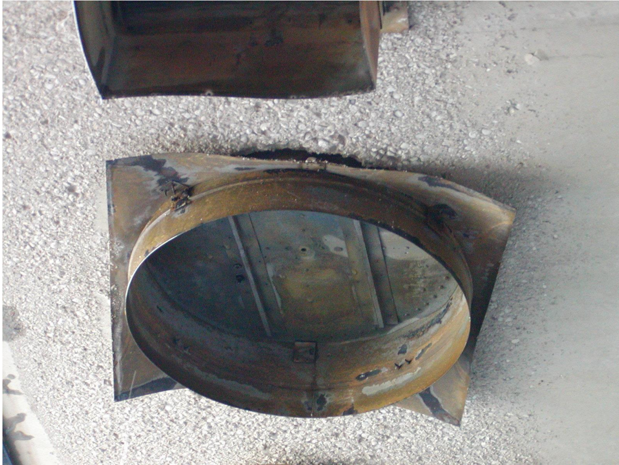
Single-blade damper after test
