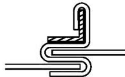
STANDING "S" ANGLE REINFORCED
