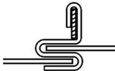
STANDING "S" BAR REINFORCED
