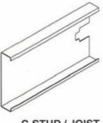
C-STUD / JOIST S-SECTIONS
