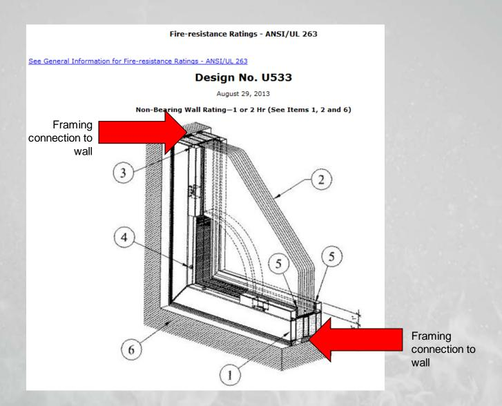
Steel Framing Members\* — Nom 4-1/4 in. (2 hr /TGP 120) and 3-1/2 in. (1hr /TGP 60) wide with lengths cut according to glazing opening size. Secured to steel studs with No. 10, 4 in. long self drilling, self tapping buglehead screws spaced nominally 18 in. OC.
