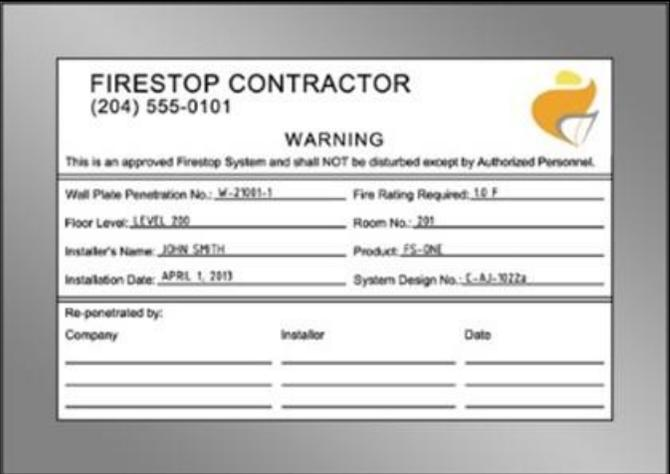
The image shows a warning label for a firestop system. It includes contact information for the contractor, a warning statement, and a table for recording re-penetration events.
