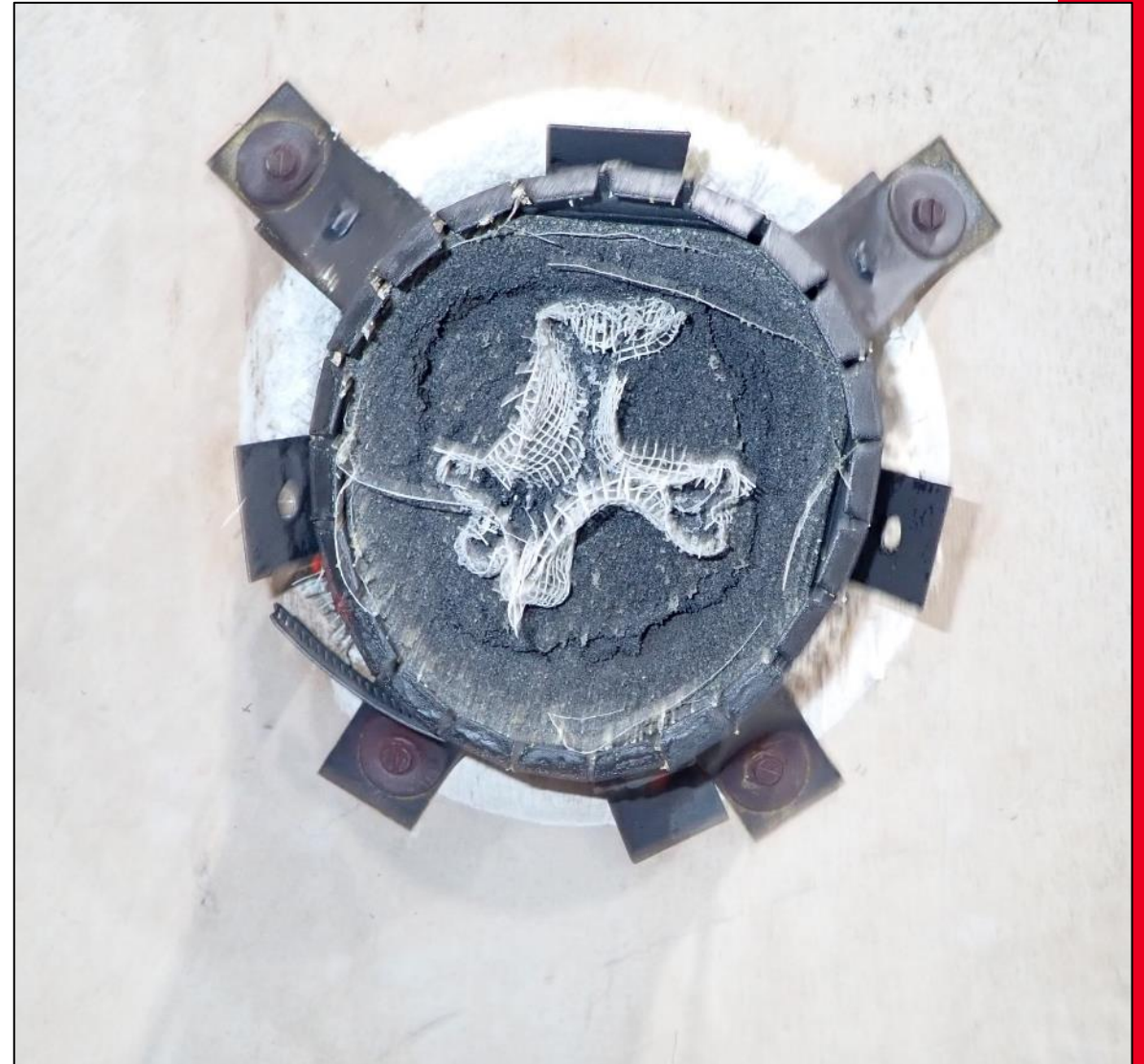
Post Test Photo of insulated Pex using Firestop Collar
